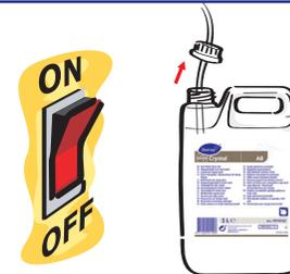
When empty: Switch off machine and wearing gloves and goggles remove feeder tube from empty container.
