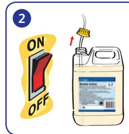
2 Switch off machine and wearing gloves and goggles remove feeder tube from empty container.
