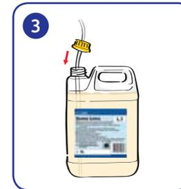
3 Wearing gloves and goggles, remove cap from new container. Place cap on empty container and dispose. Insert feeder tube into new container and secure cap.
