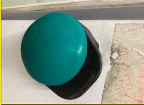
(Fig 2) No obvious signs of damage however button was not able to be depressed
