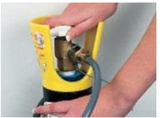
**3** Disconnect empty cylinder using only the metal spanner provided.
