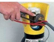
**4** Secure new cylinder in an upright position with strap or chain.
