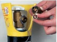
**6** Do not release the CO<sub>2</sub> or N<sub>2</sub> 40 from the cylinder to clean the valve before reconnecting.
