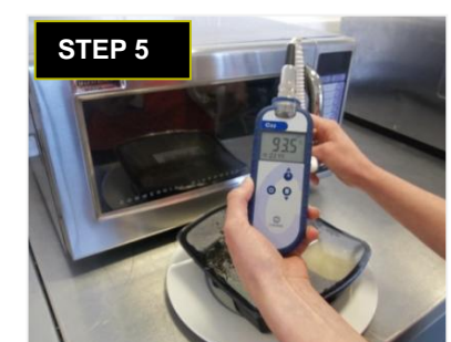
STEP 5 After cooking, leave for 30 seconds then temperature probe every meal in the main protein item. If above 82°C, record and go to Step 9
