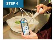
After cooking, leave for 30 seconds then temperature probe every meal in the main protein item. If above 82°C record on temperature record sheet and go to Step 7.
