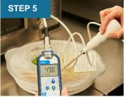
If the temperature is below 82°C, use the boost function. (30 seconds).
