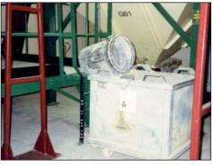
When the mini-skip was full, it was pushed to the lift, taken to ground level and lifted by fork-lift truck to empty it into a larger skip.
