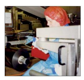
a diameter of approximately 450 mm. The machine had to be loaded a couple of times per day. The rolls were difficult to grasp, had no good hand-holds and presented a risk of finger-crushing as they were loaded onto the spindles. The spindle heights were below knee level and above shoulder level. It was a two-person lift to get the rolls into place on the spindles, and changing the rolls required the lines to be stopped, so speedy replacement was also important.
