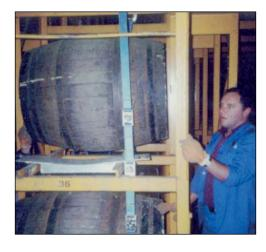
similar but even more demanding task was repositioning a cask that had turned 90° so that it was lying between and parallel to the rails. In this case the operators had to pull and lever the cask into the correct position across the rails, and also ensure that the bung was located at the top of the cask.
